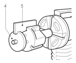
4. Insert the three wedges (5) and screw in the screws (3) completely.
