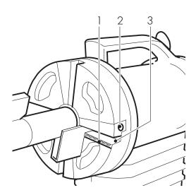
2. Tighten up the screw (2) while pressing the tool holder against the facing surface of the tool carrier at the same time.
