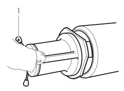
2. Advance very carefully until the first contact is made between pipe and tool. When the cutting edge of the tool machines-down over the whole circumference of the pipe, advance forwards with a uniform pressure.
