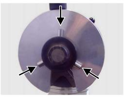
5. Attach the elbow on the mandrel and arrange it close to the straightening tool.
