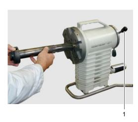
2. Attach the straightening tool (2) between mandrel and tool arbor and fix it with forward-feed supply (1).
