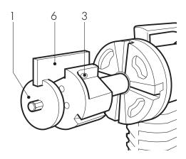
3. Insert the three wedges (6) and screw in the guiding screws (3) completely.
