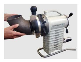
6. If the elbow is correctly positioned, tighten with the threaded spindle (4) by ring spanner (SW 18).
